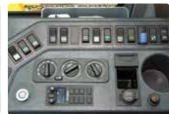
Centralized Instrument switch Panel
