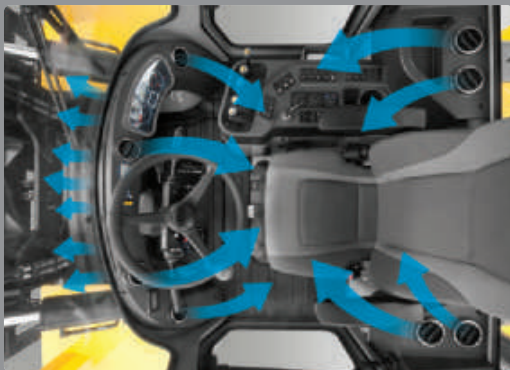
High-capacity air conditioner & heater
