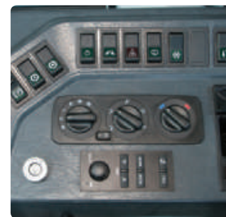
Centralized Instrument switch Panel
