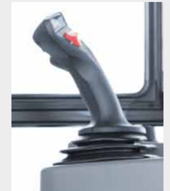
Control & operating elements: Reduced elements for intuitive operation, joystick moves ergonomically with the seat and fits any hand size
